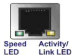
Figure 3-25: RJ-45 Ethernet Connector
